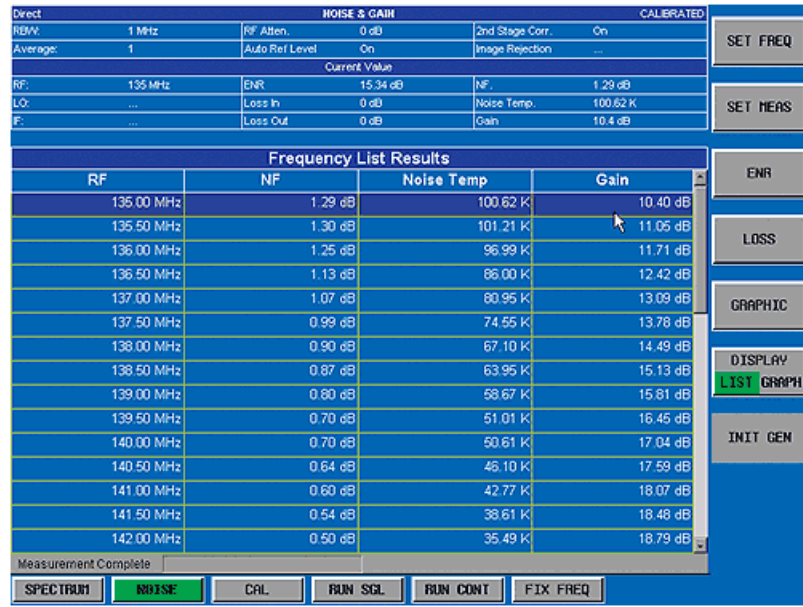
FIG 36: Tabular representation of measurements results with the R&S FS-K30 application firmware
